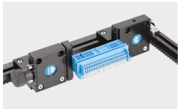
Vertically mounted spring-loaded vice without additional jaw pads, for holding flat parts of offset faces
